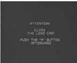
Make sure the lens cap is closed and press and hold (more than 2 sec) button M. The Correction menu appears on the screen.
