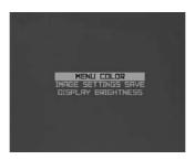
To enter the menu color menu press shortly button M. Select the color with buttons A or B and save the selected menu color by pressing and holding (more than 2 sec) button M. To exit the menu without saving press and hold (more than 2 sec) button A.
