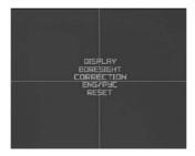
Align the reticle on the display with the scope reticle by moving the image with buttons A and B. To switch between the axis press shortly button M. Press and hold (5 sec) button M to save the alignment.
