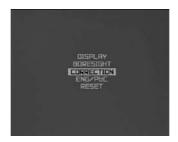
**To remove manually** the dead pixels press shortly button M to switch between X and Y. With X selected buttons A and B move the cursor horizontally, and with Y selected – vertically. Align the cursor center with the dead pixel and press and hold button M for more than 2 sec.
