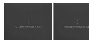
**To save** the dead pixel correction results press and hold button M for more than 2 sec with the option «Save» selected. The display shows the message confirming the successful saving.
