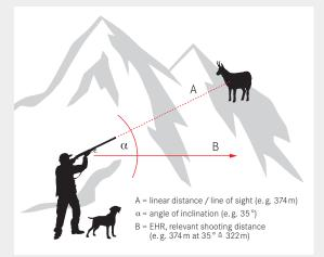
At angle shots within a range of 10 to 1,100 metres the ballistic function (EHR) calculates the relevant shooting distance from the hunter to the targeted animal. Along with linear distance and angle, the algorithm developed by Leica always takes into account arealistic ballistic curve. It also includes barometric pressure and temperature – for fast, precise and easy calculation of the right point of aim in the mountains.
